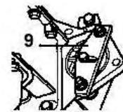
**Flywheel Locking Tool** is required on engines where the flywheel and crankshaft must be held at the correct timing position. This tool is used in conjunction with the appropriate TDC Setting Screw. After attaching the Flywheel Locking plate, the toothed profile is adjusted and locked after being fully engaged in the flywheel ring gear.
